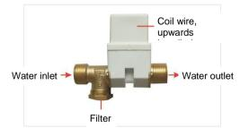
labelled on the type plate of solenoid valve is same to the voltage of power output of controller, check whether the filter of solenoid valve is completed, whether the body of valve has no damage. And during installation please pay attention to the water flow and return of solenoid valve, side with filter is the water input, water flow direction and arrow
