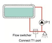
Tap seems like a remote controller, it controls the running of DHW pump. This control mode of DHW pump is an energy saving solution.
