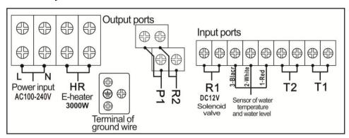
• **Power input N, L**: 20A, for power connection, L: live wire, N: zero wire, protective ground wire, please use 2mm<sup>2</sup> cable to connect the ground reliably.
