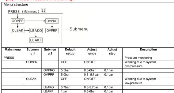
Note: The pressure monitoring function will only be available when an RPS type Grundfos Direct Sensor™ is connected.
