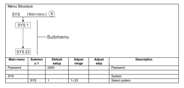
Each system has pre-programmed options and adjustments which can be activated or changed respectively if necessary. Select the system first (1-23 systems available)
