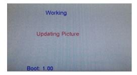
3) When upgrading is finished (depending on the size and quantity of files, running time is different), "Updating Picture OK" will show.
