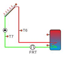
Adjust the antifreeze type and concentration of the heat transfer fluid under menu **MEDT** and **MED%**
