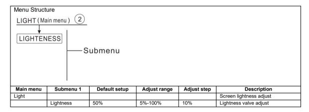
Adjust desired TFT screen lightness.
