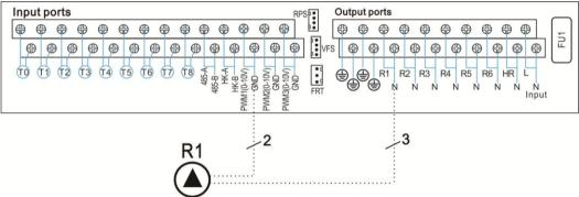
Connecting the signal wire from the high-efficiency pump
