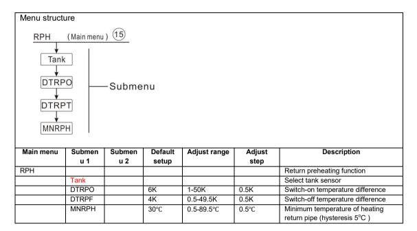
The return preheating function can be used for transferring heat from a heat source to the heating circuit return.
