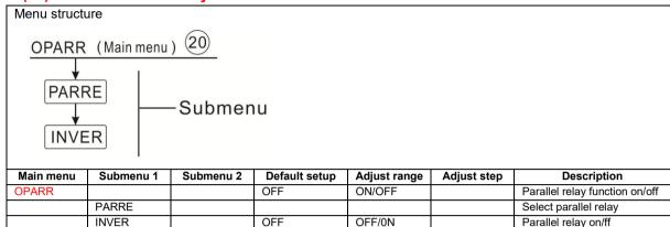
With this function, e. g. a valve can be controlled in parallel to the pump via a separate relay.
