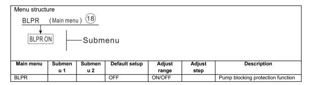
In order to protect pumps from blocking after long time standstill, the controller is equipped with a blocking protection function. This function switches on pump relays in sequence every day at 12:00 a.m. and every pump runs for 10 s at 100 % speed.
