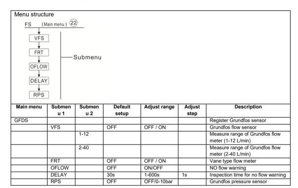
Under this menu, the Grundfos direct sensor (VFS, RPS) can be activated or deactivated, and its measurement range can be set.
