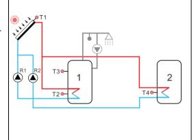
Priority heating logic will ensure to heat tank 1 firstly.
