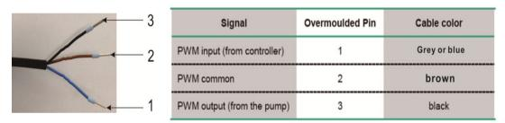
Signal wire 1 from the high-efficiency pump is connected to GND port of controller Signal wire 2 from the high-efficiency pump is connected to PWM port of controller Signal wire 3 from the high-efficiency pump is not connected to the controller Some pumps connections are available as above, for example:
