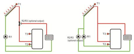
Collector heat transferring valve logic
